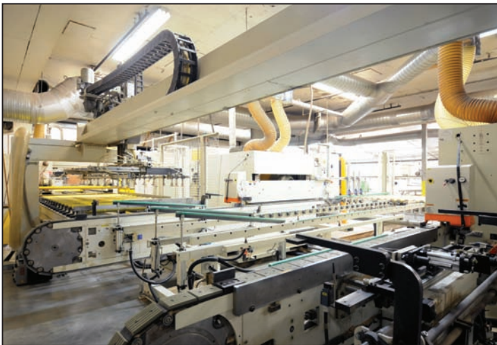
MAHROS RUNNER/D-C vacuum feeder/stacker
