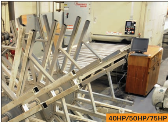
TIMESAVER 51" wide belt sander & carousel sheet flipper
