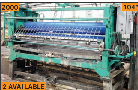
BLACK BROTHERS 22D 1175 CTR 104" top & bottom glue spreader
