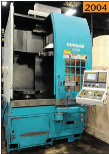
DOOSAN V740 CNC vertical lathe
