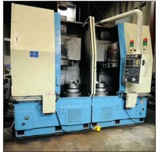
HWACHEON ECO-5V 2SP twin spindle CNC vertical lathe
