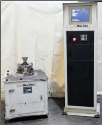
MICRO-POISE 3687 stiff pivot balancer with MP9400 computer
