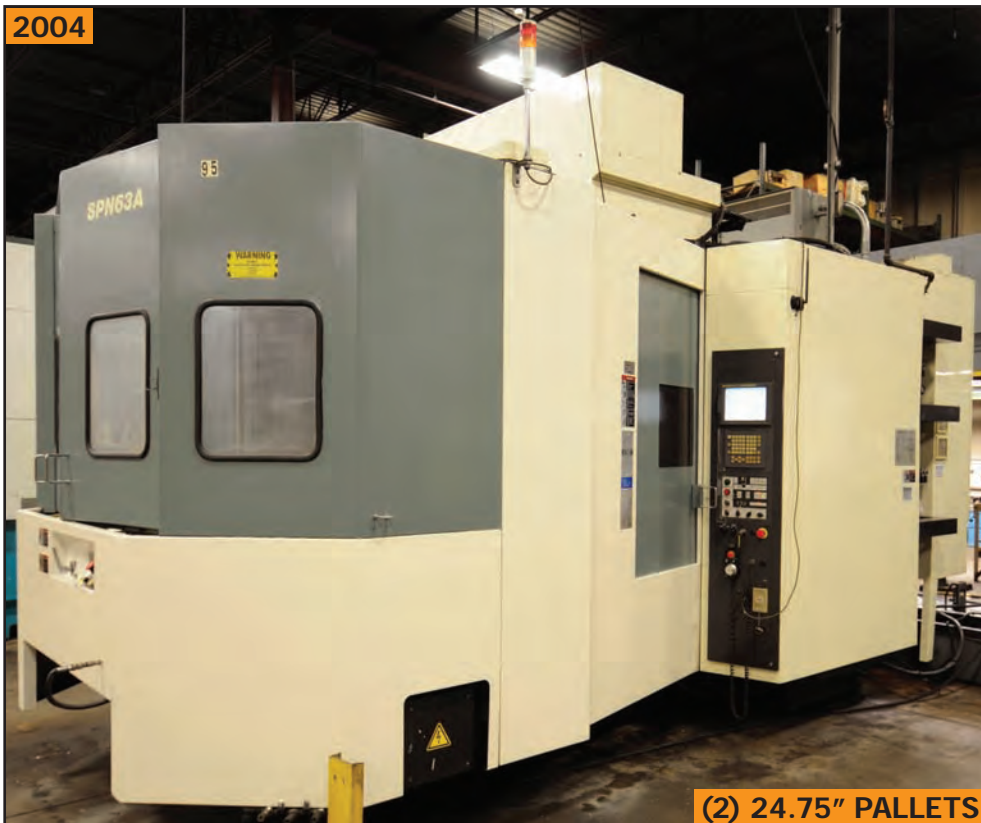
NIIGATA SPN63A CNC 4 axis twin pallet horizontal machining center
