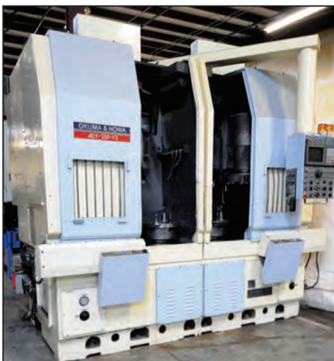
OKUMA HOWA ACT 2SP V3 twin spindle CNC vertical lathe
