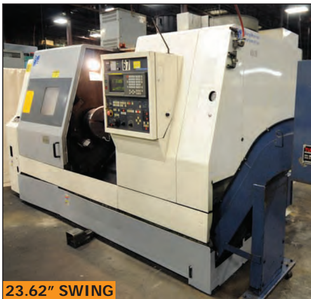
MORI SEIKI SL-35B/750 CNC turning center
