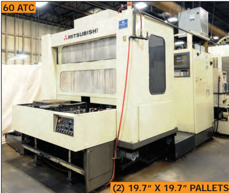
MITSUBISHI M-H50D CNC twin pallet horizontal machining center
