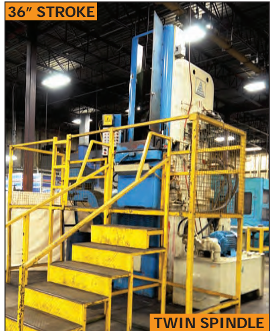
APEX vertical broach with chip conveyor
