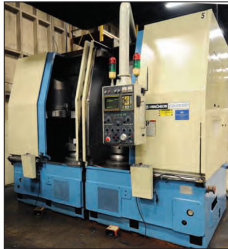
HWACHEON ECO-5V 2SP twin spindle CNC vertical lathe
