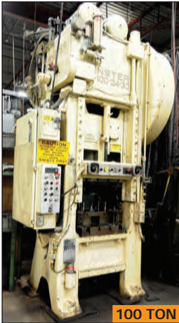
MINSTER S1-100-24-30 mechanical straight side press
