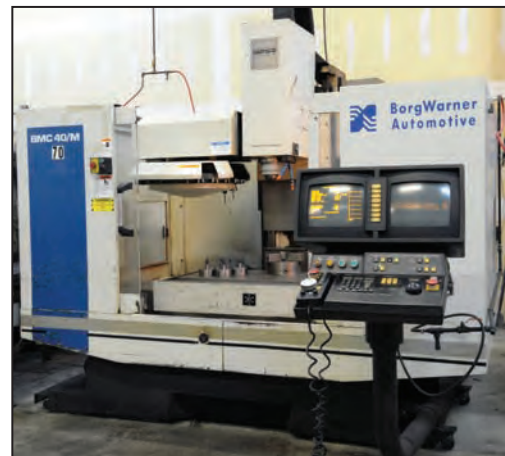
HURCO BMC 40M CNC vertical machining center
