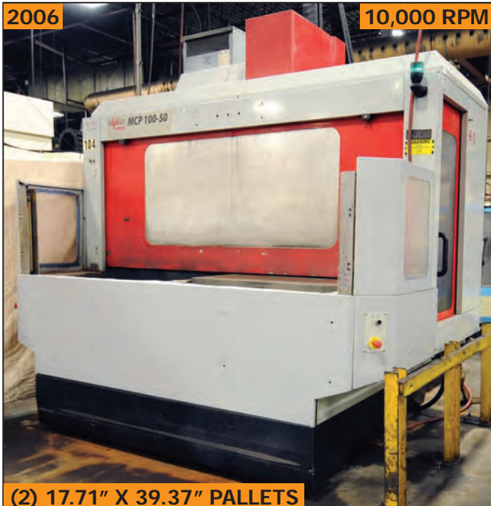
(2) 17.71" X 39.37" PALLETS FAMUP MCP100-50 CNC twin pallet vertical machining center
