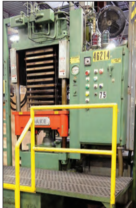
DAKE 27-56S hydraulic thermal platen press
