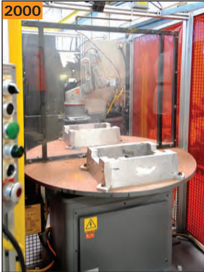
2000 MOTOMAN robotic welding cell
