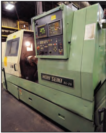
MORI SEIKI SL-25B/750 CNC turning center
