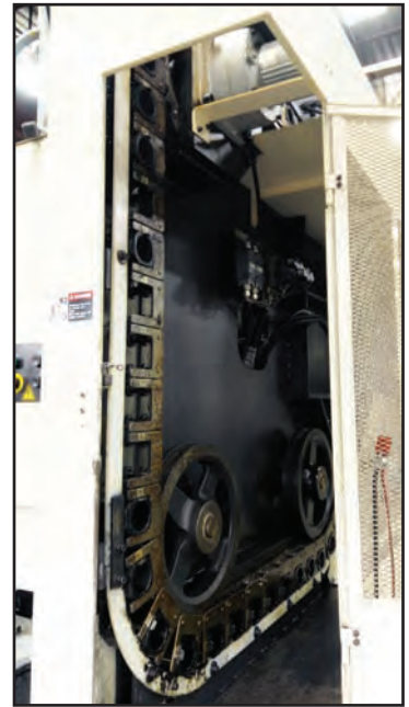
View of NIIGATA 60 station ATC
