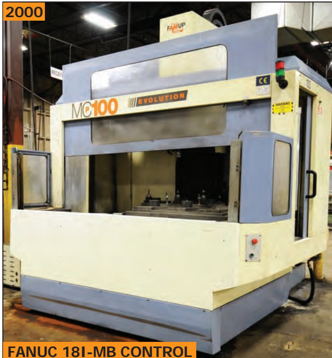
FANUC 18i-MB CONTROL FAMUP MCP100E CNC twin pallet vertical machining center
