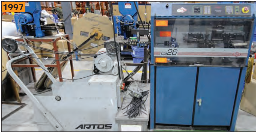
1997 ARTOS CS-26 single conductor, round cable wire cutting and stripping machine
