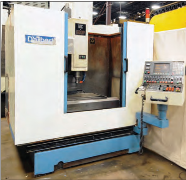
MITSUBISHI MC-500P CNC vertical machining center
