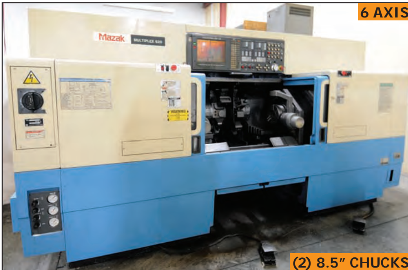
MAZAK MULTIPLEX 620 6-axis, double opposed spindle CNC turning center
