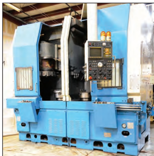
DOOSAN DOOTURN 2SP-3V twin spindle CNC vertical lathe
