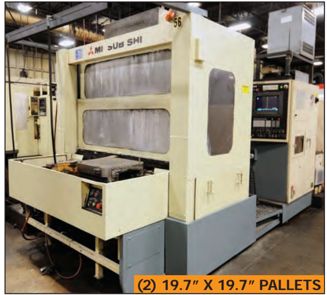
MITSUBISHI M-H50C CNC twin pallet horizontal machining center
