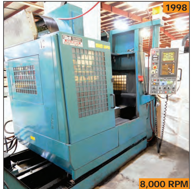
MATSUURA RA-IIF CNC twin pallet vertical machining center
