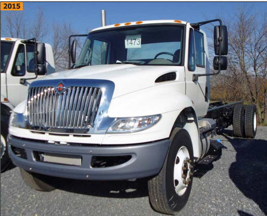
INTERNATIONAL (2015) 4300 SBA 4X2 Single axle truck with CUMMINS ISB 240 240hp diesel engine, EATON SYNCRO 6 manual transmission, cruise control, a/c, air ride driver seat, 275 miles, VIN # 3HAMMMMN0FL720098 TRUCK # 1473
