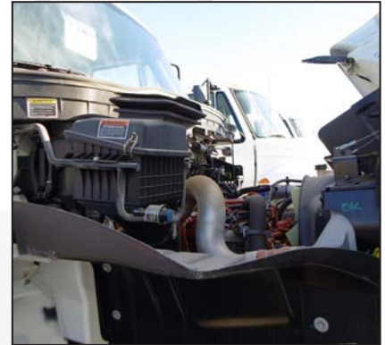
INTERNATIONAL (2015) 4300 SBA 4X2 Single axle truck with CUMMINS ISB 240 240hp diesel engine, EATON SYNCRO 6 manual transmission, cruise control, a/c, air ride driver seat, 260 miles, VIN # 3HAMMMMN2FL720099 TRUCK # 1475
