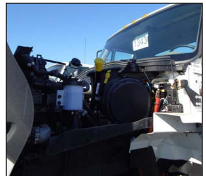
INTERNATIONAL (2015) 7600 SBA 6X4 2010 Tandem axle truck with NAVISTAR N13 430hp diesel engine, EATON/FULLER 8 speed manual transmission, power windows & locks, cruise control, a/c, air ride driver seat, 172 miles. VIN # 1HTGSSNT6FH181416, TRUCK #1343
