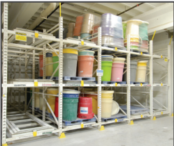
Partial view of rollout racking
