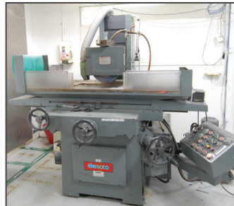
BEMATO BGM3060AH hydraulic surface grinder
