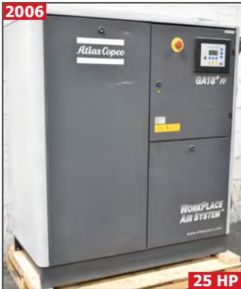
ATLAS COPCO GA18+ 25 HP rotary screw air compressor
