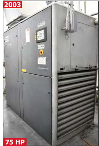
ATLAS COPCO GA55 75 HP rotary screw air compressor
