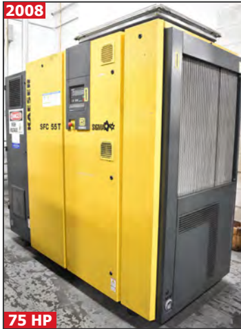
KAESER SFC 55T 75 HP rotary screw air compressor
