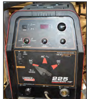
LINCOLN ELECTRIC portable digital TIG welder
