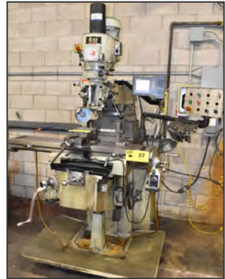
FIRST LC-VS vertical turret milling machine
