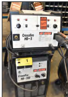
CROSSFIRE HD-350 portable digital MIG/ARC welder
