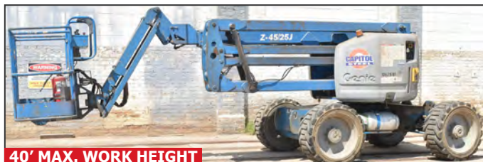
GENIE Z45/25J IC POWER 4x4 articulating boom knuckle lift
