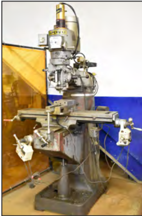
SUPERMAX VC-1-VS-T vertical milling machine
