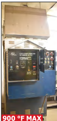
900 °F MAX WELD ENGINEERING electric rebake oven
