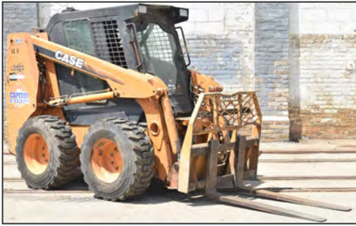
CASE 440 wheeled skid steer loader
