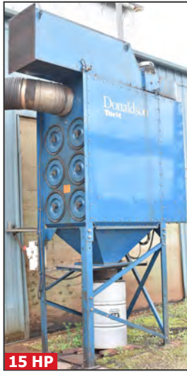
DONALDSON-TORIT DFT3-12 cartridge-type dust collector
