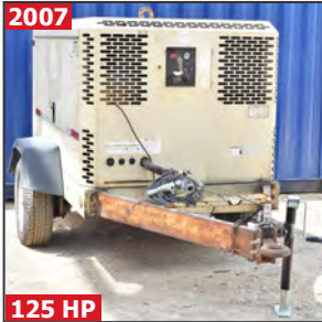
INGERSOLL-RAND VX0375 single axle tow-behind air compressor
