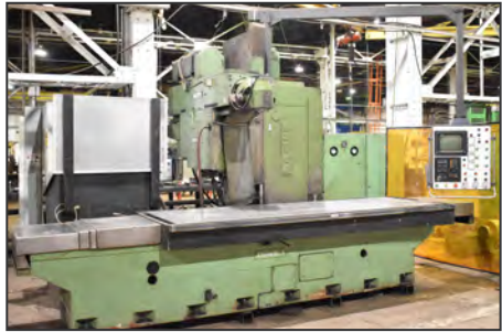
ZAYER BF-3000 bed-type CNC universal milling machine
