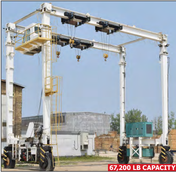
DROTT 650B outdoor diesel mobile gantry
