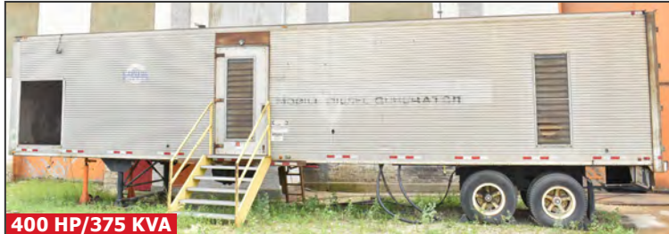
BBC mobile diesel generator system with enclosed tandem-axle trailer
