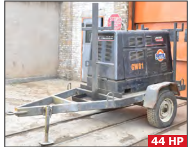
LINCOLN ELECTRIC COMMANDER 400 d single axle tow-behind generator/welder
