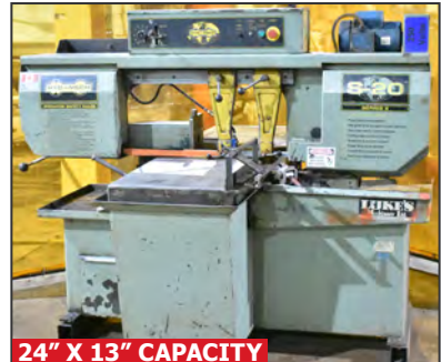
HYD-MECH S-20 SERIES II horizontal band saw
