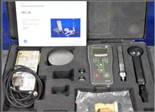
GE INSPECTION TECHNOLOGIES MIC 10 UCI portable digital hardness tester
