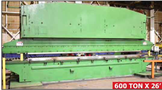
BEYELER 600T 600-ton capacity hydraulic press brake
