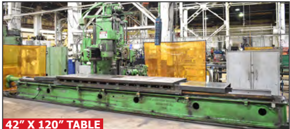
ROCKFORD-PONTIAC open sided bed-type vertical/horizontal hydraulic planer mill
