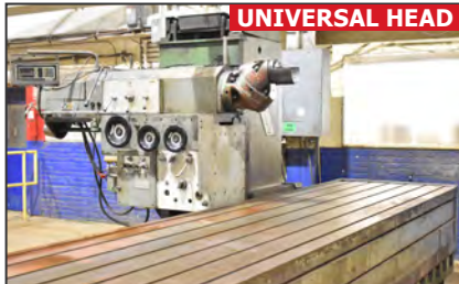
BUTLER ELGAMILL CS-10 bed-type milling & boring machine
