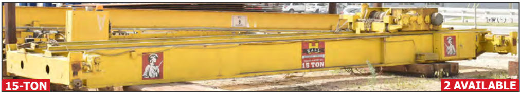
HALL SENTRY capacity double girder top-running overhead bridge crane
