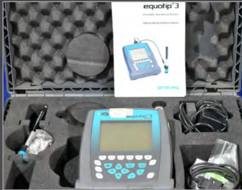
PROCEQ EQUOTIP 3 portable digital hardness tester
