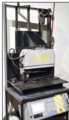
MECCO/COUTH MC2000 dot peen marking system
