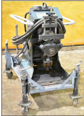
GULLCO GBM-18 portable automatic plate beveling machine
