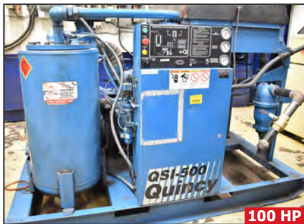
QUINCY QSI-500 100 HP skid-mounted rotary screw air compressor
