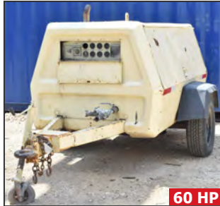
INGERSOLL-RAND P185WJD single axle tow-behind air compressor
