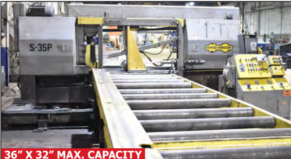
HYD-MECH S-35P automatic horizontal band saw
