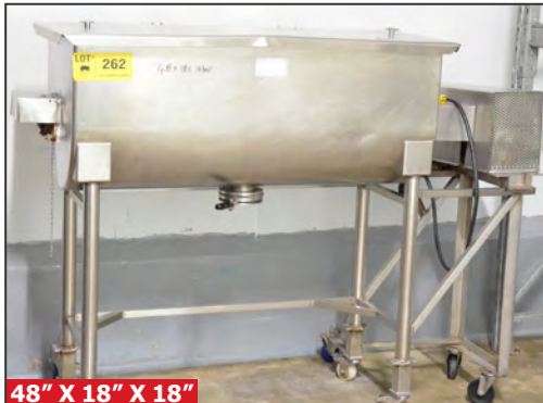
AMERINOX single shaft stainless steel portable ribbon blender
