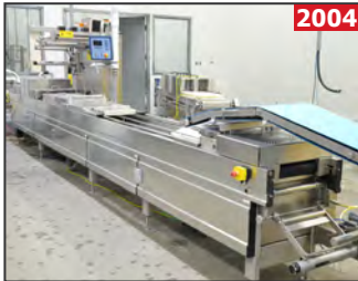
MULTIVAC R530 horizontal automatic rollstock form fill thermoformer
