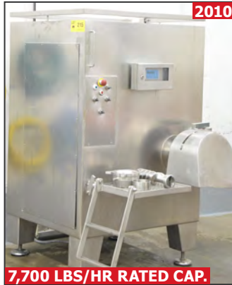
SEYDELMANN WOLFGRINDER AM130/3 stainless steel mixer grinder
