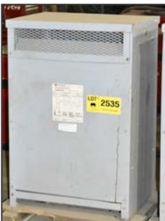
CUTLER-HAMMER 75 KVA transformer
