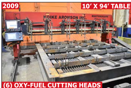
2009 KOIKE ARONSON MASTERGRAPH MILLENIUM SERIES MGM3100 CNC gantry-type oxy-fuel burning table
