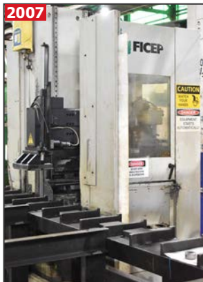
FICEP VICTORY 1101DX CNC structural beam drilling line
