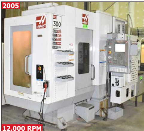
HAAS EC 300, high-speed CNC twin pallet horizontal machining center
