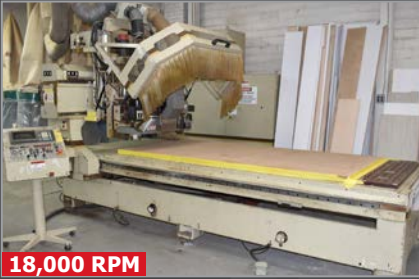
18,000 RPM ANDERSON STRATOS WFD CNC router
