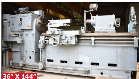
LEBLOND MODEL 3220 heavy duty custom sliding gap bed engine lathe
