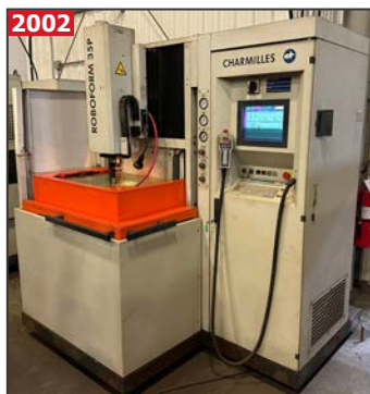
CHARMILLES ROBOFORM 35P CNC wire EDM w/ CNC control, pendant control, 16" x 20" table, travels: X - 13.7"; Y - 9.8"; Z - 13.7", work tank dimensions 24" x 40", 1,760 lb. max. workpiece weight, s/n: 1-5443/641205
