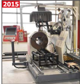
QSPR CNCPCR-42A CNC pipe profile plasma cutting machine
