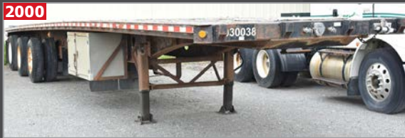
MANAC 10448 48' tri-axle flat deck trailer
