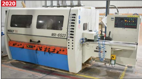
HOLYTEK MX-6S23 6-head side moulder
