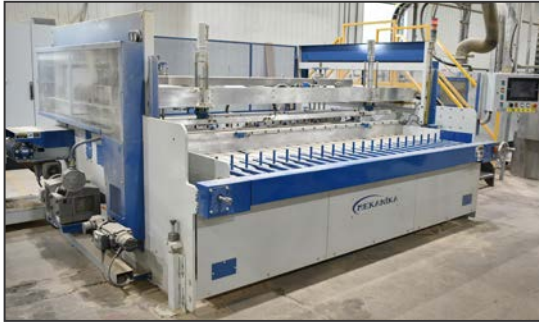
MEKANIKA NG-014 sander infeed transfer system
