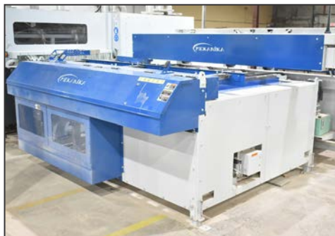
MEKANIKA NG-002 vacuum loader
