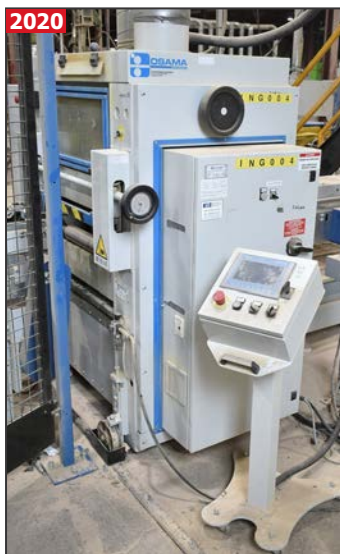
OSAMA GSHM-3-400 hot melt roller coater
