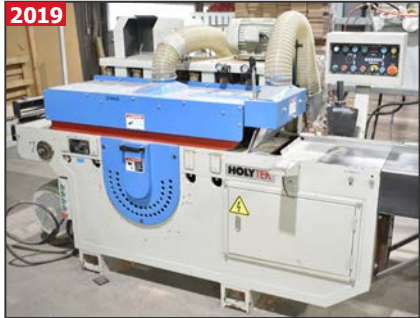
HOLYTEK GRS300A multiple edger
