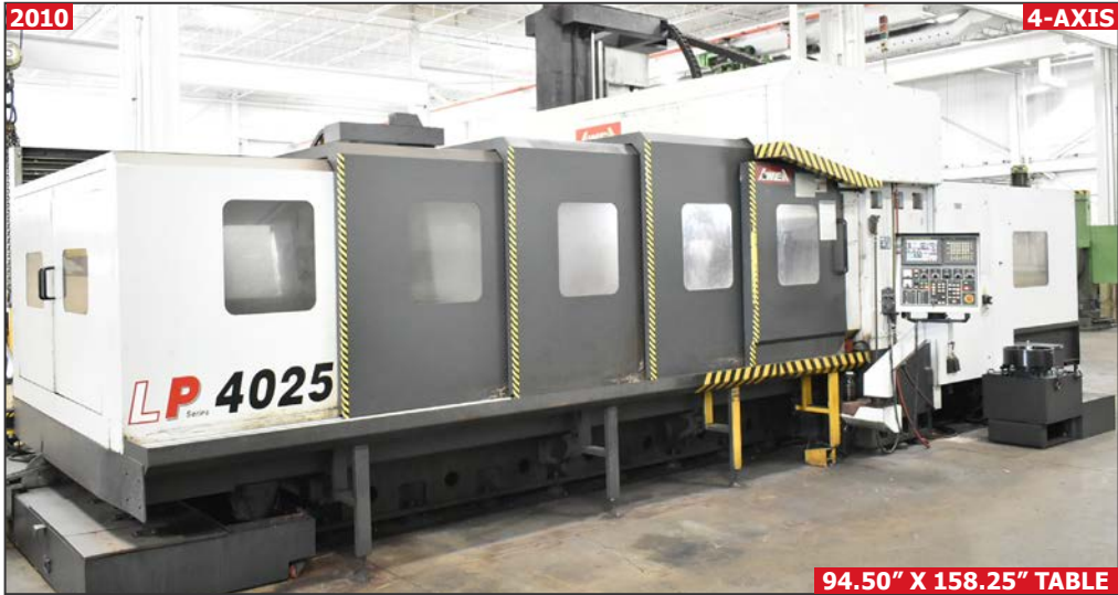
AWEA LP4025 CNC 4-axis bridge type vertical machining center
