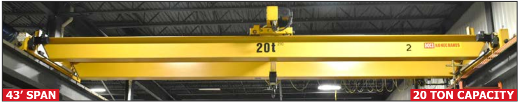
KONE double girder top running overhead bridge crane
