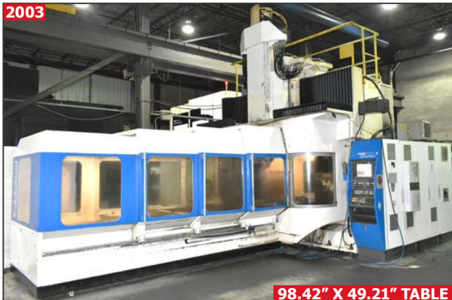
HURON KX200 5-axis high speed bridge type CNC vertical machining center
