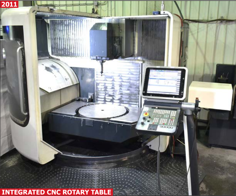
DMG DMU 100 MONOBLOCK 5-axis high speed universal machining center
