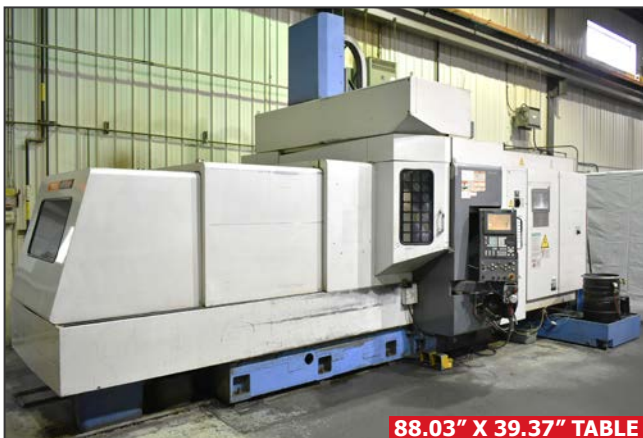
MAZAK FJV 50/80 high speed bridge type CNC vertical machining center
