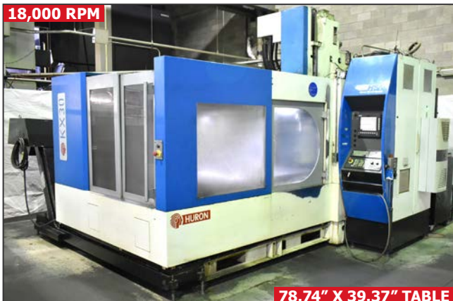
HURON KX30 high speed bridge type CNC vertical machining center
