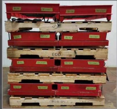
Partial view of battery roller stands
