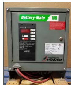
AMETEK 600M112G 24-volt battery charger
