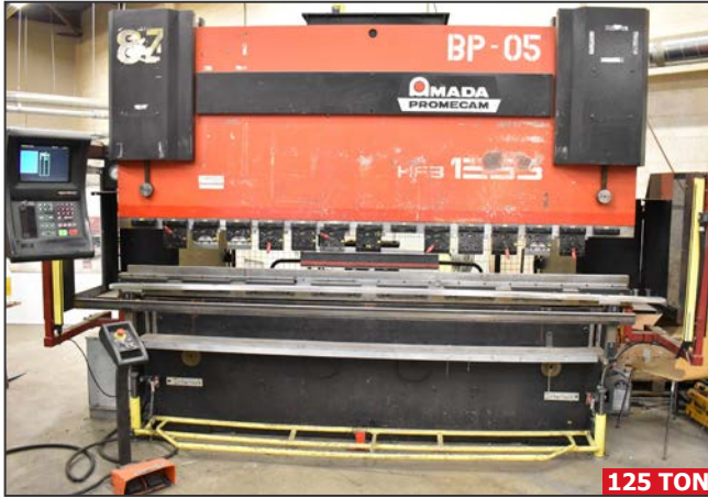
AMADA PROMECAM HFBO 125 TON CNC 10' hydraulic press brake
