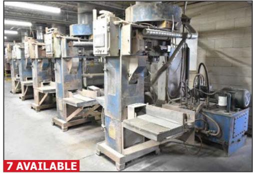
Partial view of hydraulic pre-form presses
