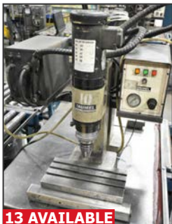
TAUMEL T251-8126 bench type automatic orbital rivetter
